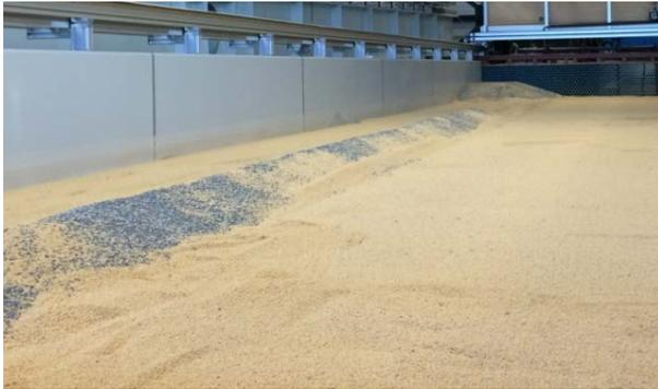
Figure 3. Scale model of the upstream section of a longitudinal training dam (1:60) in a 2.5-metre-wide flume in the Kraijenhoff van de Leur Laboratory for Water and Sediment Dynamics in Wageningen.
